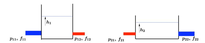
Logical choice of inputs: the pressures  $p_{11}, p_{12}, p_{21}, p_{22}$ , and of outputs: the flows  $f_{11}, f_{12}, f_{21}, f_{22}$  $(h_1, h_2$ : state variables)
